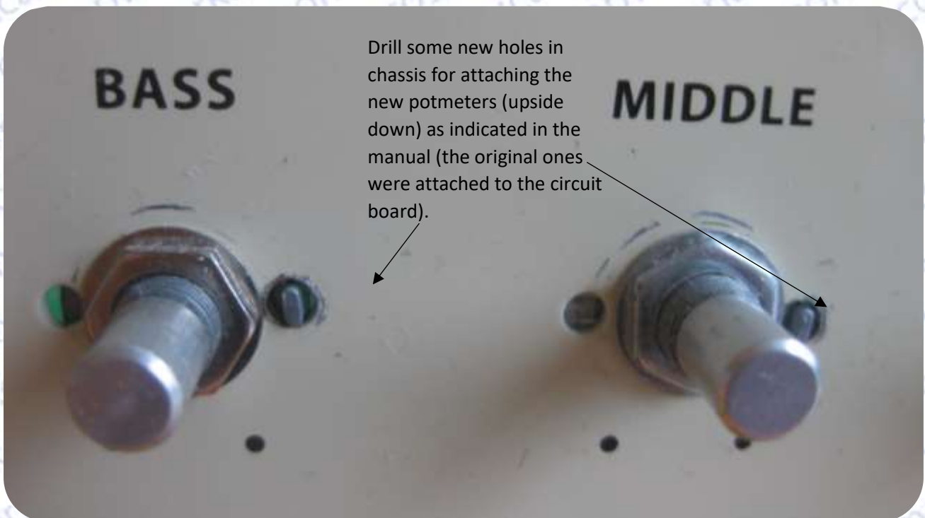
Figure 17 Drill some new holes in chassis for attaching the new potmeters
