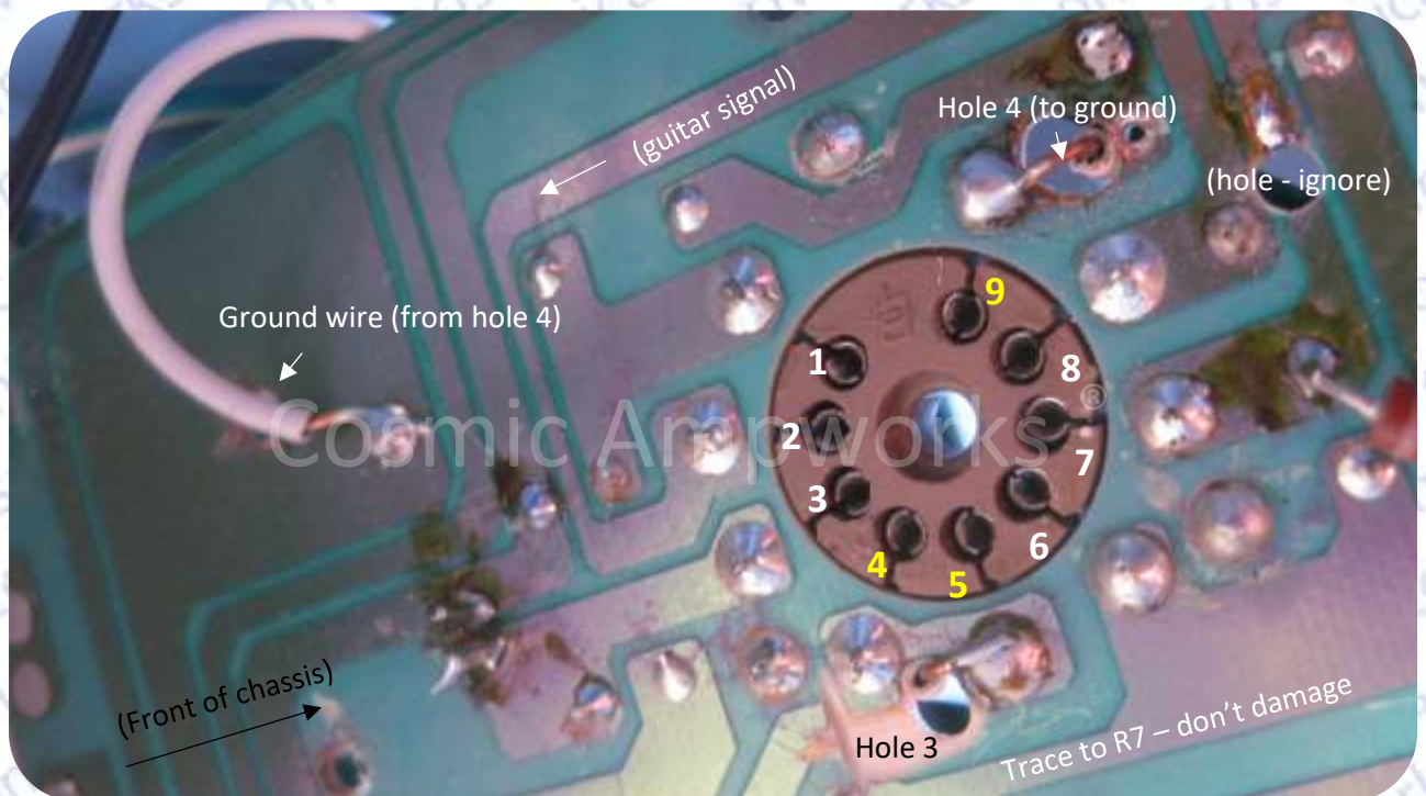
Figure 23. Drill two holes near the first preamp tube: Drill hole 3 right next to the tube socket solder connections of pins 4 and 5; make sure not to damage the trace running from pin 6 of the tube (anode) to R7 (load resistor). Drill hole 4 just above the tube socket solder connections of pin 9. Make sure not to accidentally damage the wire bridge on top of the board! Ideally, also interrupt the circuit board trace in go, because the heater traces spread hum throughout the circuit in their stock layout. Use the green wire for the heater supplies (picture actually show whpite/grey wire).
