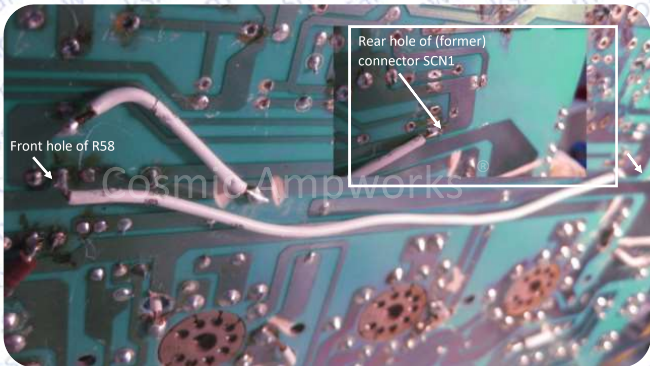
Figure 30. Re-establish ground connection for components to the right of C15 with a wire between the front hole of (the former) R58 and the rear hole of the removed connector SCN1. The ground connection will be needed for the new volume control (see further down).
